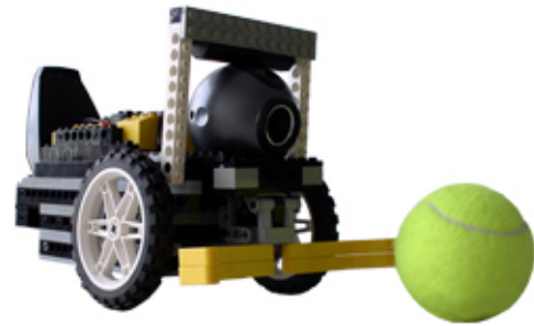
Fig. 1. SoccerBot : 2-independent-wheel-drive Lego® Mindstorms™ robot mounted with Logitech® QuickCam® Pro 5000.
