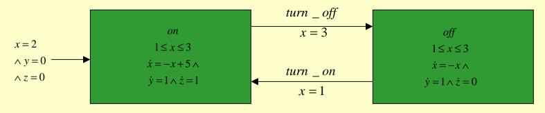
Thermostat automaton augmented for safety verification
