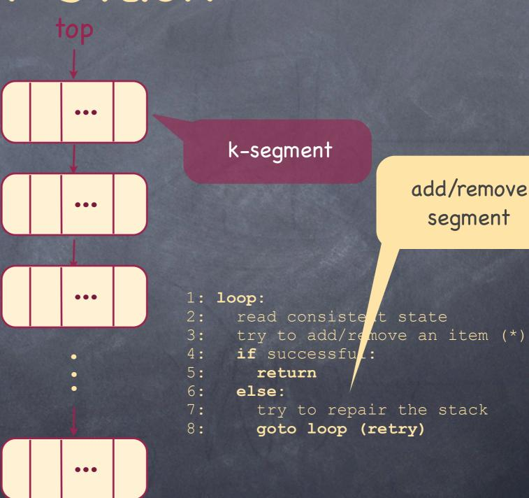
lock-free = non-blocking k-segment add/remove segment 1: loop: read consistent state try to add/remove an item (\*) if successful: CAS - based return 6: else: try to repair the stack 8: goto loop (retry)
